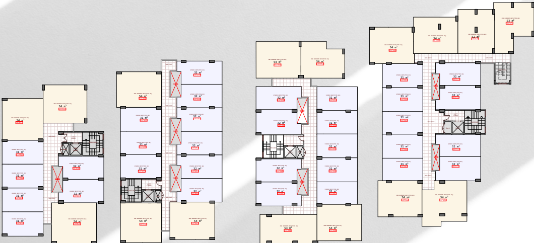
UNIT FLOOR AREAS BLOCK A - FLOOR AREA 427.58 m 2 TYPICAL FLOOR PLAN ONE BEDROOM UNIT - 3 NO. STUDIO UNIT - 6 NO.
