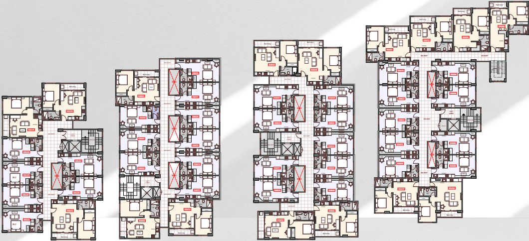
FURNITURE LAYOUT BLOCK A - FLOOR AREA 427.58 m 2 TYPICAL FLOOR PLAN ONE BEDROOM UNIT - 3 NO. STUDIO UNIT - 6 NO.
